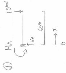
$$\begin{aligned} \sum Y = V_A - 10 &= 0 \quad \therefore V_A = 10 \text{ kN} \\ -M_A &= -10 \times 4 \quad \therefore M_A = 40 \text{ kNm} \\ M_x &= -40 + 10x, \quad Q_x = (M_x)' = 10 \end{aligned}$$
